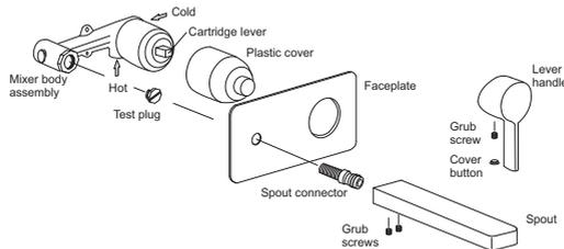
5. Fit the lever handle assembly to the cartridge lever and tighten the grubscrew through the access hole(2.5mm allen key). Fit the cover button to conceal the access hole.
